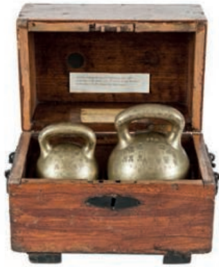
27 A CASED SET OF "COUNTY OF WESTMEATH LOCAL STANDARD" DUMBELL BRASS WEIGHTS BY NICHOLL & FOWLER, LONDON, one weighing 14 pounds, the other 28 pounds, each stamped 'County of Westmeath' and stamped numerously with monarch's initials 'VR' and 'ER', contained in a fitted hinged top mahogany box, with side brass handles.
